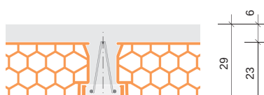
strop Porotherm 23/50/6 strop Porotherm 23/62.5/6
